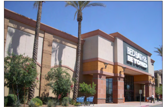
Large building mass should be broken by varying wall surfaces, roof heights, and change in texture and materials.
