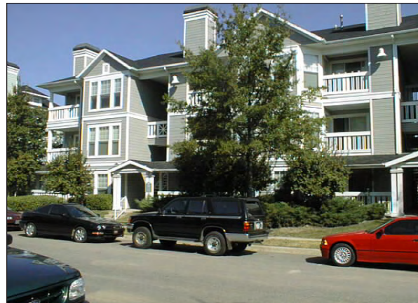
Larger building facades should be broken with overhangs, changing roof lines, and other design elements that provide shadows and depth to the building façades.
