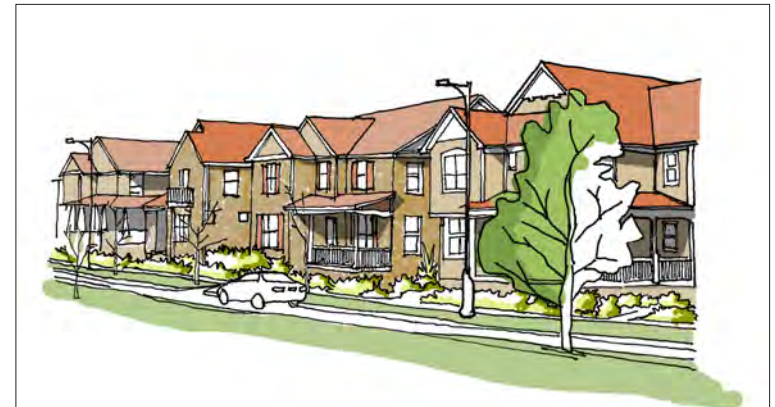
Exhibit A.4.6: Building mass may be broken up by projecting or recessing the walls of the front façade.
