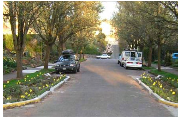
Vegetated curb extensions with cuts to allow stormwater retention may be designed in bulb-out parking areas.
