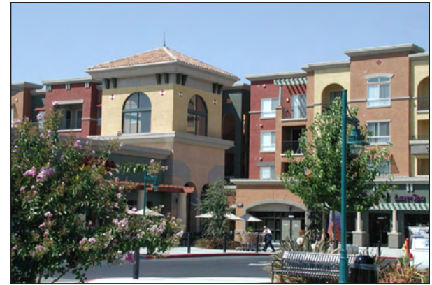
Windows, entries, and doors should occupy maximum wall space at pedestrian level.
