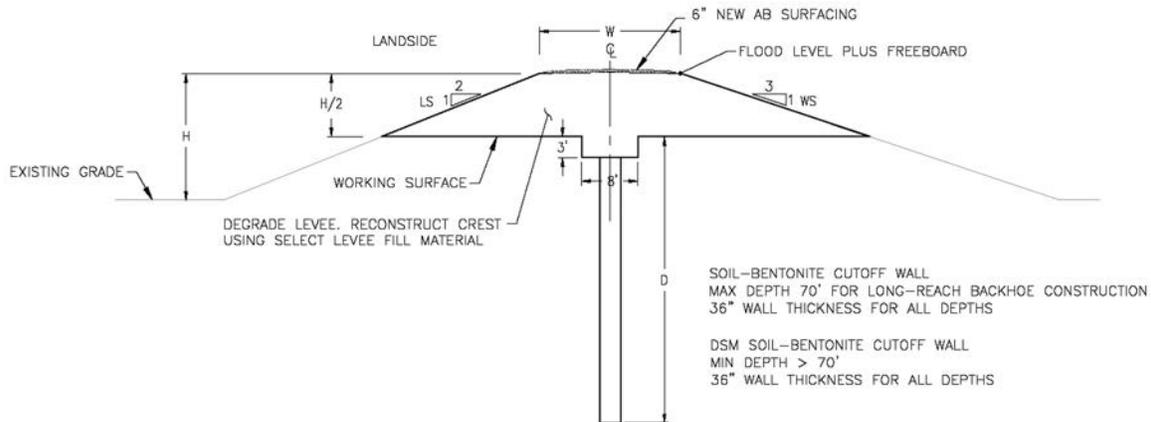
An interlocking sheetpile system could be used in lieu of a SB cutoff wall. The interlocking sheetpile system would be installed through the levee crown with minimal levee degrade. The wall alignment along the levee crown could be trenched 2 to 3 feet to allow driving the top of the sheetpiles below the levee crest.
