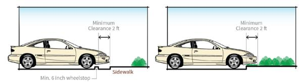
Figure 1500-20-2: Curb Stops and Clearance
